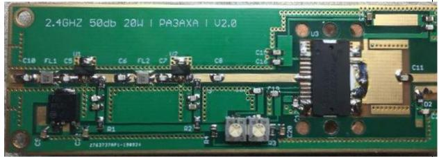
Place the heats spreader and pcb on a flat surface. The sides of the enclosure will fit the pcb (the side with the 3 holes on the output side!). Solder first left and right next to the input and output trace. (see photo below). Make a few more soldering spots to keep the enclosure sides in its shape. It is not necessary to solder it all around.
